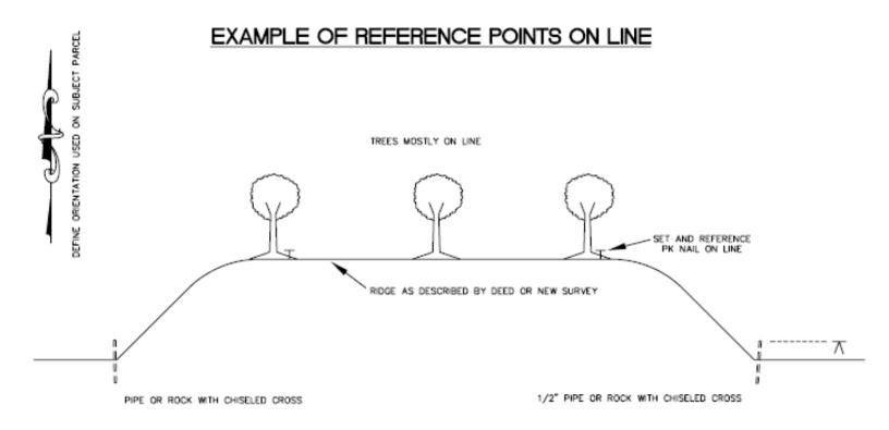
SET AS MANY POINTS AS WOULD BE NECESSARY ON RIDGE LINES (THAT REPRESENT EXISTING OR PROPOSED BOUNDARY LINE)
