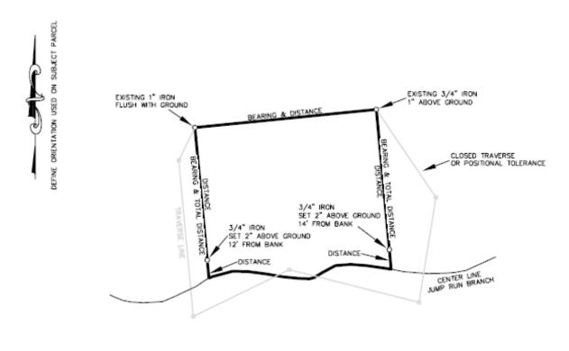
SURVEYOR MUST PERFORM CLOSED LOOP FOR RATIO OF PRECISION
